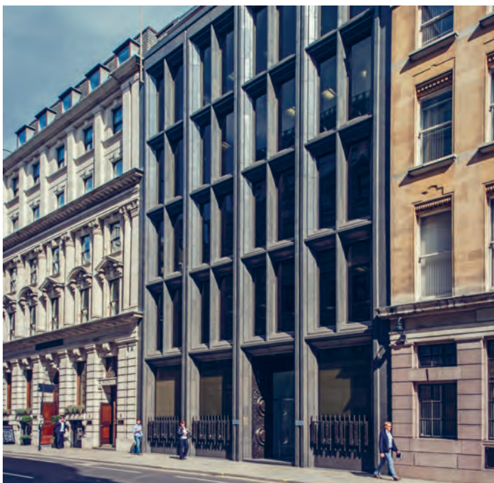
Harmonious: similar scale and facade rhythm to neighbouring heritage buildings using high quality materials and not imitating heritage styles- fits into the street
