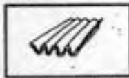
Corrugated sheet metal - How the typical roofing material. Use of a low slope (Shore's) material combined with proper fasteners - usually screws with washers - usually greatly improves metal roof performance during hurricanes.
