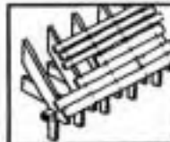
Sheathing for wooden purlins or beams. Modern plywood makes an effective replacement. Ideally, 3/4 inch or 1 inch thick plywood improves roof performance during storms. Also see appropriate fasteners.
